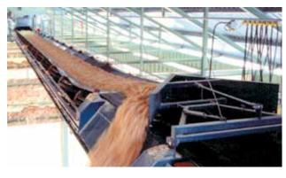
**Idler roller conveyors** are used for bulk goods such as chips, sawdust, bark, etc. Low energy consumption, silent operation and low maintenance cost. Available in several sizes up to 900 cu.m. per hour.
