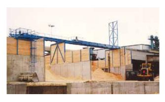
**Scraper conveyors** can be 600 mm to 1800 mm wide, designed for material transport in the upper or lower part, and up to 80 degrees inclined, All versions are intended for reliable, heavy duty operation at low operating cost.
